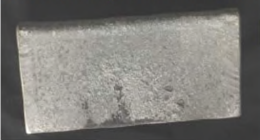
Extruded tube from permanent immersion zone
