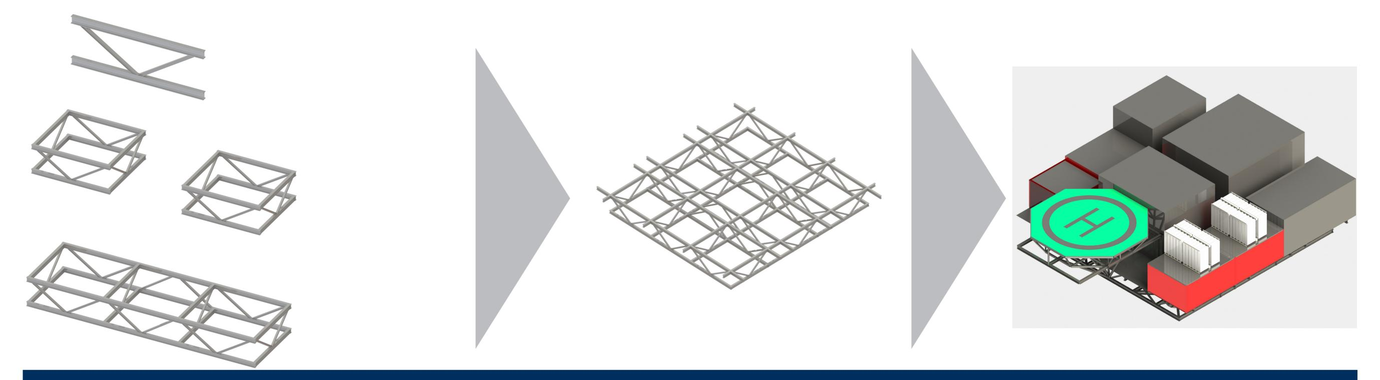
Development of a multi-purpose topside design. A modularised and standardised as well as scalable multi-purpose topside design is developed, that can additionally be customized according to side specific requirements. Customisation up to a certain degree allows consideration of different, very specific platform requirements depending on site conditions and power processing requirements.
