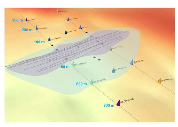
**Plume monitoring:** Array of 14 platforms with 29 optical and acoustic sensors quantifying sediment particle concentrations in the bottom water
