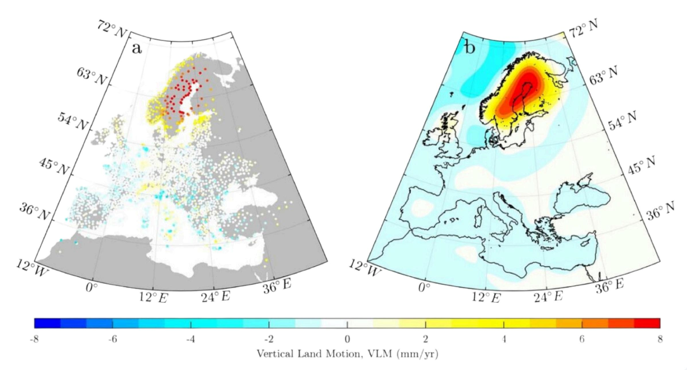
(a) Preferred filtered and smoothed present day VLM field from Piña-Valdés et al. (2022) and based on data from ~4000 GNSS stations in Europe.
